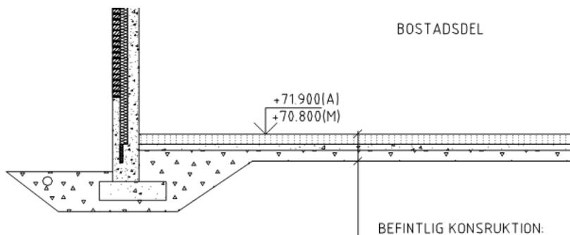
Figure 2 Original construction of floor in Alingsås bottom floor flats
