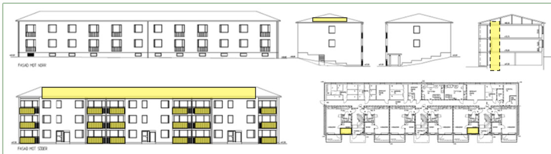
Figure 1 Location in building for PV cells (on roofs and balconies) and elevator wells.
