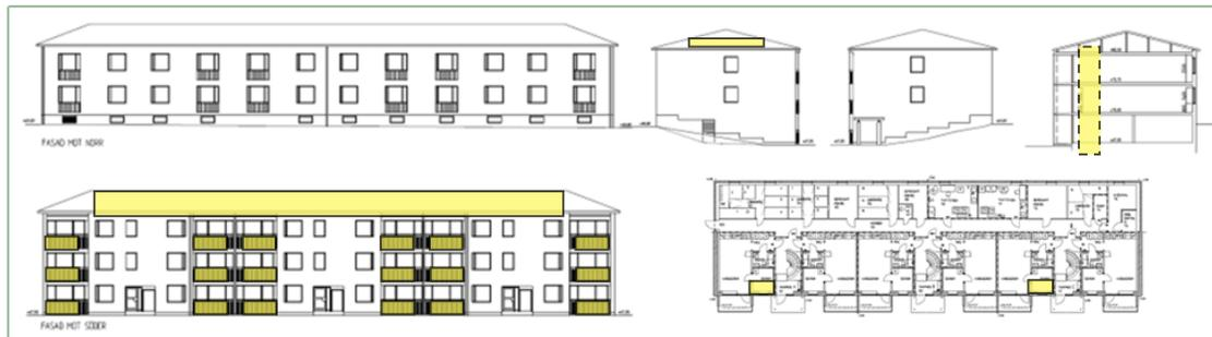
Figure 1 Location in building for PV cells (on roofs and balconies) and elevator wells.
